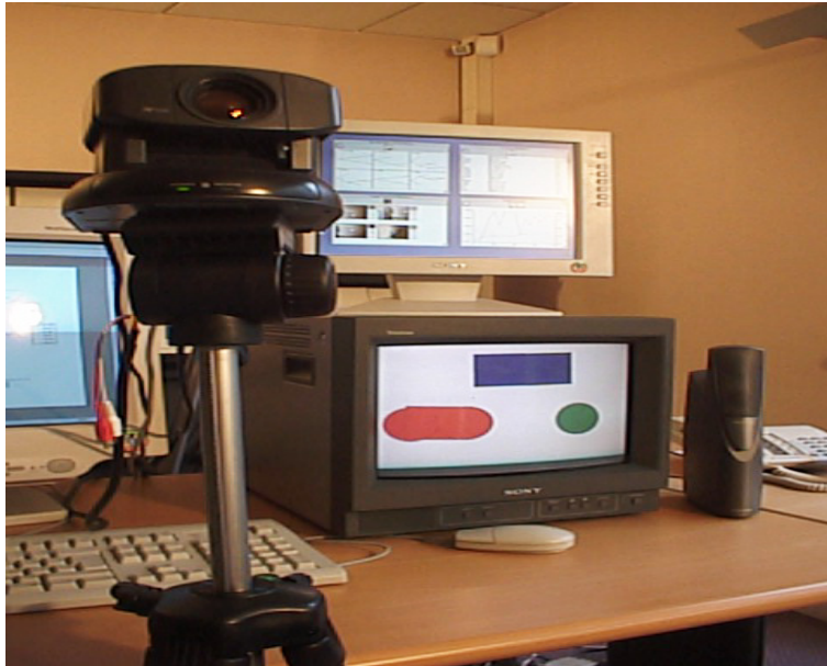
Figure 1: Picture of one 'Talking Head' being a steerable camera capturing images about scenes with geometrical figures in front of them. The captured image is shown on a separate monitor.
