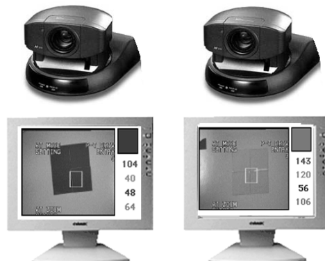
Fig. 1. Two Talking Head cameras and associated monitors showing what each camera perceives.
