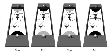
**Fig. 1.** The four environments  $E_{10}$ ,  $E_{01}$ ,  $E_{00}$ , and  $E_{11}$ .  $L_1$ ,  $L_2$  and  $L_3$  refer to the lights. The revolving door is indicated by the horizontal bar in the centre of the arena. In each environment, the arrows indicate the direction in which the door revolves. The cylinders with spikes on the white floor represent the robots.
