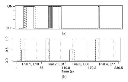
**Fig. 4.** Post-evaluations of group  $g_4$ . Dashed lines refers to the robot placed at the beginning of trial 1, in the upper side of the arena; continuous lines refer to the robot placed in the lower side of the arena. (a) Sound signals. (b) Floor sensors readings. Dotted line indicates the state of  $L_3$ , 1 = ON, 0 = OFF. On the x axis is indicated the time of start and end of each trial.
