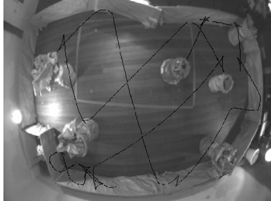
Figure 3: A typical example of wandering behavior in the arena resulting from a parallel combination of forward movement and obstacle avoidance. Behavior of robots could be monitored by an overhead camera and tracking programs.
