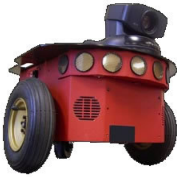
Figure 1 The Pioneer robots used in the RatSLAM and RatChat projects have cameras, laser sensors, sonar sensors, and odometer sensors with which to explore the world. In simulations with RatSLAM, the robots have a wandering behavior to build up a map of the world.
