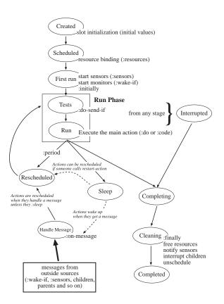
Figure 4: Process Flow in Tapir.
