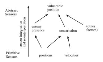
Figure 2: Raw sensor data is transformed into more complex concepts via the abstract sensor hierarchy.
