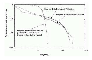
Figure 7: Degree distribution of the nodes in  $V_C$  for both PlaNet<sub>syn</sub>, PlaNet, and when the model incorporates no preferential attachment; for PlaNet<sub>syn</sub>,  $\epsilon = 0.0701$  and the results are averaged over 100 simulation runs
