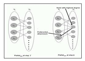
Figure 6: A partial step of the synthesis process. When the language  $L_4$  has to connect itself with one of the nodes in the set  $V_C$  it does so with the one having the highest degree (=3) rather than with others in order to achieve preferential attachment which is the working principle of our algorithm
