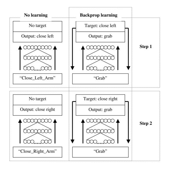
Fig. 3. The procedure that implements the grounding transfer from two basic action words to a combined action word consists of multiple steps, one for each basic word involved. Each of these steps is composed of a feed-forward phase, during which a desirable output is computed, and a learning phase, during which this output is used as a target input for backpropagation learning. Input patterns are binary representations of words, while output patterns are forces applied to each motorized joint.
