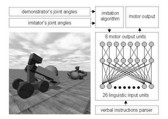
Fig. 1. Functional organization of the robotic model. The picture (bottom left) shows the 3D simulation environment with the demonstrator and imitator robots. The diagram on the right describes the linguistic input from the parser to the neural controller, and the corresponding motor output. The imitation algorithm compares the demonstrator's joint angles with those of the imitator.
