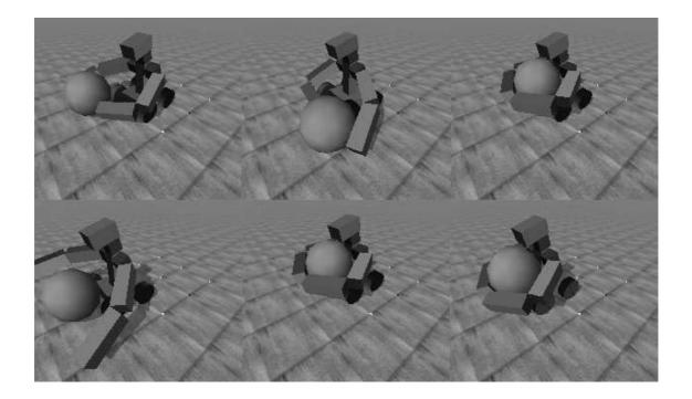
Fig. 2 - Two example sequences for the acquisition of higher-level behaviors HG1 (top row) and HG2 (bottom row). Top row (from left to right): "GRAB is CLOSE\_LEFT\_ARM and CLOSE\_RIGHT\_ARM" (BG & BG = HG1). Bottom row: "CARRY is MOVE\_FORWARD and GRAB" (BG + HG1 = HG2).
